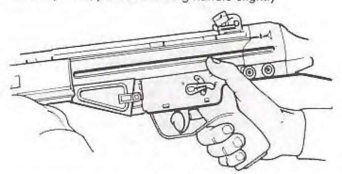
rearward and rotate it downward out of the retaining notch; then release the handle to allow it to return to its original position. Then point the muzzle in a safe direction, rotate the selector lever to "F" or "Fire" and depress the trigger to allow the bolt to return to its closed or fired position. Rotate the selector back to "Safe" before proceeding.
